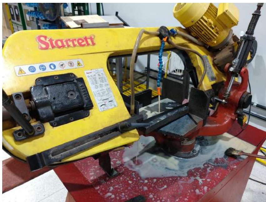
Figure 4.7. Starrett S3720 bandsaw during cutting procedure.
